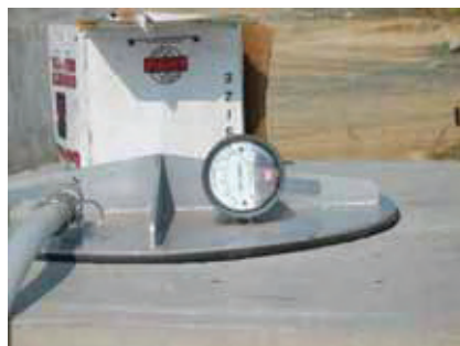
10 inches of Hg applies a load of 720 psf to Winchester Building Supply septic tank.
