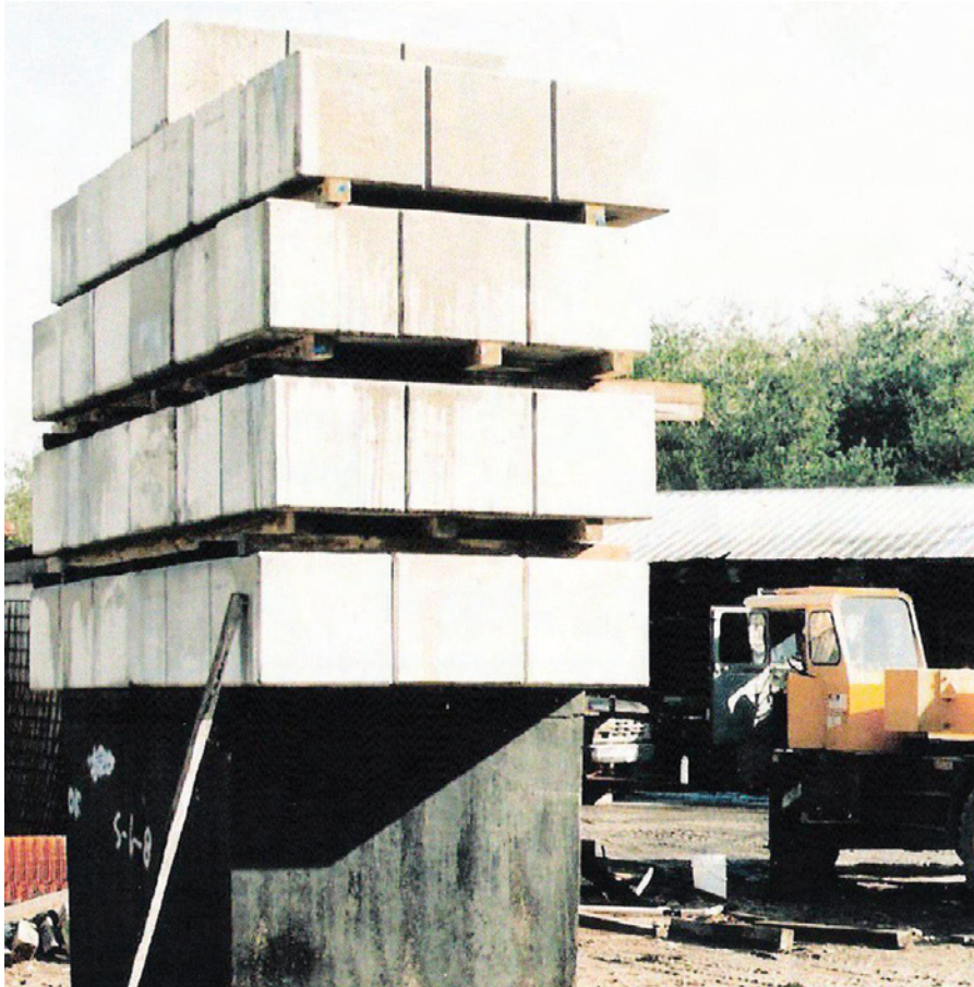
Diehl Vault, Orangeville, Pa., loads septic tank with 77,500 lbs. on top. A 22-inch vacuum could load the top just as much, but it would also load the sides.
